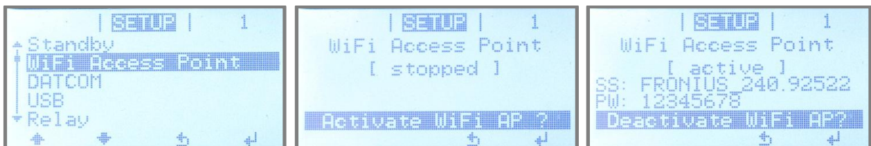
Fig.1: Activating the WiFi access point on the Inverter's display - Setup menu
